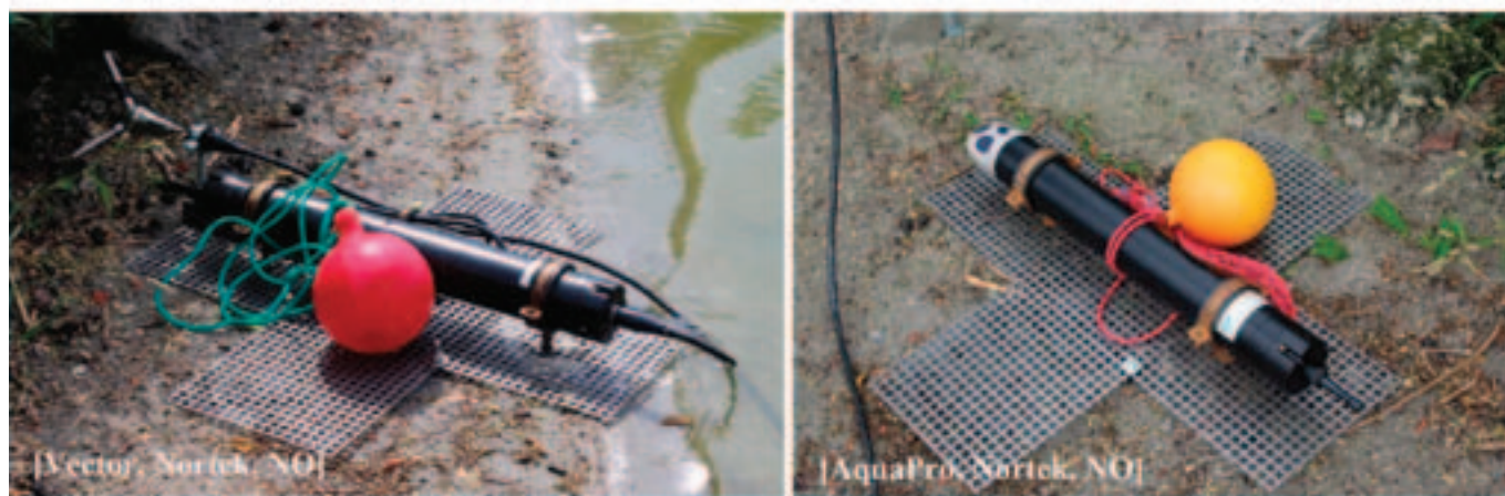
Figure 5. Doppler instruments for measuring hydrodynamics in study-site (ADV, left) and (ADCP, right)
